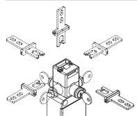
The head can be quickly turned to each of the four sides of the switch by unfastening the two fastening screws.
