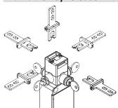
The auxiliary key release device is used to allow the maintenance or the entry into the machinery to authorized personnel only. Turning the key corresponds to actuating the solenoid: the actuator is released. The device can be turned, thereby enabling installation of the safety switch in the machine while the release device remains accessible on the outside of the guard.
