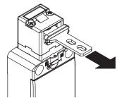
The robust interlocking system guarantees a maximum actuator holding force of  $F_{1max} = 1100 \text{ N}.$
