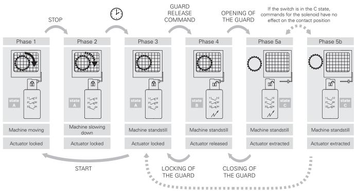
CLOSING THE GUARD with a de-energised solenoid causes the switch to move to the B state and then to the A state in quick succession
