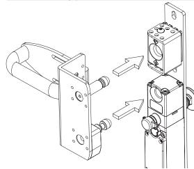
When closing the guard, the upper metal pin attached to the handle plate hits the bottom of the centering block (A) before the actuator hits the switch housing, leaving a safe distance (B) to avoid collisions between the devices
